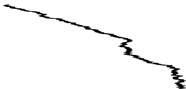
FIG. 3. An aggregate composed of 500 particles using only 0D, 1D, and 2D staggers. The exclusion of 3D and 4D staggers leads to the formation of a ribbon like morphology.
